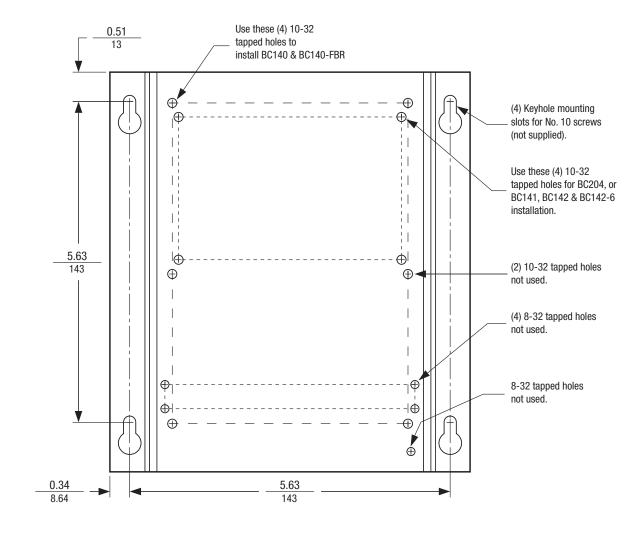
**Notes: 1.** Always mount heat sink in vertical position (if possible) to achieve maximum efficiency. **2.** (4) 10-32 screws are provided. **3.** Install with keyhole slots in position as shown.
