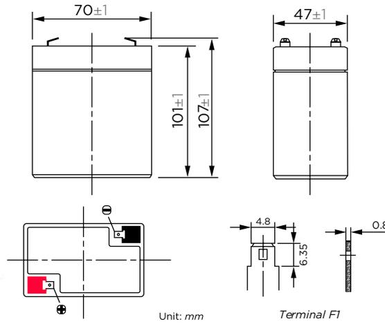
These rechargeable batteries are lead-lead dioxide systems. The dilute sulfuric acid electrolyte is absorbed by separators and thus immobilized. Should the battery be accidentally overcharged producing hydrogen and oxygen, special one-way valves allow the gases to escape thus avoiding excessive pressure build-up. Otherwise, the battery is completely sealed and is, therefore, maintenance-free, leak proof and usable in any position.
