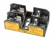
Specifications Description: Class CC fuse blocks for use with Class CC fuses (Cooper Bussmann LP-CC, KTK-R, and FNQ-R). Dimensions: See Data Sheet 1105 Poles: 1 to 3 Ratings: Volts: — 600V Amps: — 1/0-30A SCCR: — 200kA RMS Sym. Agency Information: CE, UL Listed (Guide IZLT, File E14853), CSA (Class 6225-01, File 47235) Flammability Rating: UL 94V0
