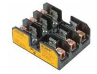
Specifications Description: Supplementary fuse blocks for use with any <sup>1</sup>%<sup>2</sup>" x 1½" fuses (Cooper Bussmann® KTK, FNQ, FNM, BAF, PV, and AGU). Dimensions: See Data Sheet 1104 Poles: 1 to 3 DIN Rail Adapters: See page 413 for DRA-1 & DRA-2 Ratings: Volts: — 600Vac/dc Amps: — <sup>1</sup>/<sub>0</sub>-30A SCCR:— 10kA RMS Sym. Agency Information: CE, UL Recognized (Guide IZLT2, File
