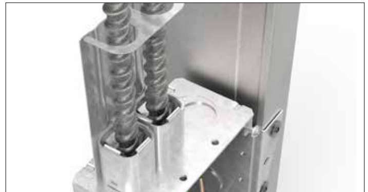
Step 5. Slide cable management up and snap into the box and Quick-Lok connector after all cables are installed.
