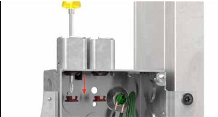
Step 2. Pop out the plug by inserting a screwdriver through the top of the Quick-Lok connector in the location where cable will be installed. If you accidentally pop out too many plugs, you can reinstall.
