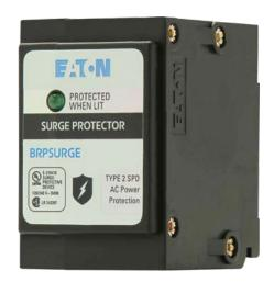
Type 2 surge products are permanently connected devices that are installed on the load side of the service entrance overcurrent protective device, including surge protective devices (SPDs) located at the branch panel. These devices can be used as replacements for what were previously known as secondary surge arresters. Eaton's Type 2 surge protective modules are NEC® 230.67 compliant as well as UL® 1449 and cUL® listed. They are tested to the highest industry standards for ultimate safety.
