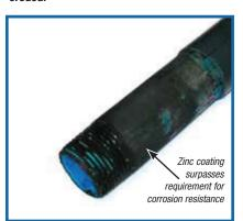
The purpose of the Preece test is to evaluate the zinc coating on galvanized rigid conduit to ensure adequate protection from corrosion per UL6.2.2. The test will also determine if the surface of the conduit has been damaged as a result of preparation for PVC coating.
