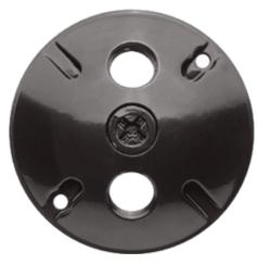
Die cast round covers with one or three 1/2" holes. Fit 4" round boxes. Supplied with thick foam rubber gasket and two #10-24 stainless steel screws. 3 hole cover comes with one die cast 1/2" close-up plug.
