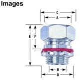
**Download Photo Image** Dimension A in Inches: .950-1.050 Dimension B in Inches: 1.050 Dimension C in Inches: 1.730 Dimension D in Inches: 1.500 Dimension E in Inches: 1-7/8 Dimension F in Inches: 13/16
