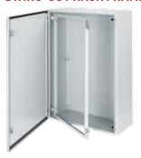
Swing-Out Rack Frames provide 120-degree swing-out access for 19-in. rack equipment. Welded rack frame mounts to front flange. Distance from frame to door surface is 1.32 in. [33 mm] for solid doors and 1.07 in. [27 mm] for window doors. Frame is painted white. Mounting hinge and latching hardware provided. Order separately clip nut package catalog number XNM5 and screws XSM5 (metric) or AN1032 and screws AS1032 (English). Swing-Out Rack Frame cannot be mounted on adjustable mounting kit.
