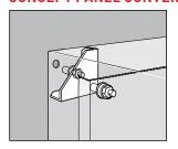
Panel Conversion Kit adapts enclosure for mounting standard NEMA-style panels in CONCEPT enclosures. Bracket attaches to rear collar stud. Kit includes four adapter plates and hardware for mounting panel.
