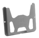
Data Pockets provide convenient storage for wiring diagrams, operation manuals and other documentation inside an enclosure. Pocket mounts on studs located on the inside of a solid-door enclosure. Constructed of high-impact thermoplastic, pockets are dark gray and have cutout areas for easy access and visibility to contents. Mounting hardware included.
