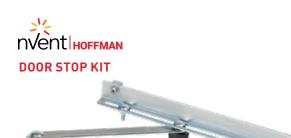
Door Stop Kit secures the door in the open position. Kit can be installed at the top or bottom of a door which opens horizontally. Door opening angle can be easily adjusted by means of a wing nut. Stop arm slides neatly out of the way when the door is closed. All parts are plated. Mounting hardware included.
