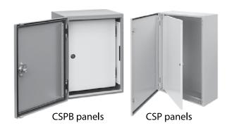
Panels swing clear from the front of the enclosure to provide access to mounted internal equipment. For CSPB panels, maximum swing is 94 degrees. For CSP panels, maximum panel swing is 106 degrees. Distance from panel surface to door when in the latched position is 1.71 in. [43 mm] for solid doors and 1.45 in. [37 mm] for window doors. Kits include panel, brackets and hardware to mount to the front flange. Panel is painted white.
