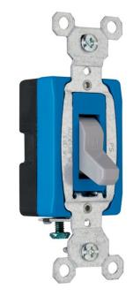
Construction 1pole Switch, Back & Side Wire, 15amp 120/277 volt, Gray.
