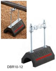
DBR Series Adjustable Height Base with two (2) ½"-13" Electro Zinc All Threaded Rod Risers and a B3114-3½" Pipe Roll with Sockets Dimensions - Overall Height as Specified Base - 4" High (101mm) x 6" (152mm) Wide x 9.6" (244mm) Length (base length)
