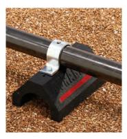
Dimensions - 4" (101mm) High x 6" (152mm) Wide x 9.6" (244mm) Long (base length) Ultimate Load Capacity - (uniform load) \* DBP - 500 lbs. (2.22kN) DBM - 200 lbs. (0.89kN)
