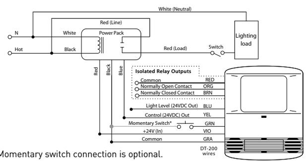
\*Momentary switch connection is optional. Connect only when momentary switch is installed.
