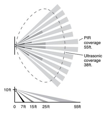
Coverages shown are maximum and represent half-step walking motion. Under ideal conditions with no barriers or obstacles, coverage for half-step walking motion can reach up to 2000 ft<sup>2</sup>, while coverage for typical desktop activity can reach up to 1000 ft<sup>2</sup>.
