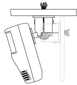
A swivel mounting bracket attached to the sensor allows the sensor to be angled for wall or ceiling mounting.
