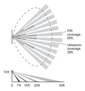
Coverages shown are maximum and represent halfstep walking motion. Under ideal conditions with no barriers or obstacles, coverage for half-step walking motion can reach up to 2000 ft<sup>2</sup>, while coverage for typical desktop activity can reach up to 1000 ft<sup>2</sup>.
