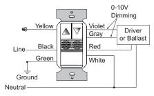
Note: Requires Class 1 wiring for 0-10V dimming.
