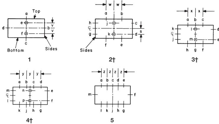
\*Drilling and tapping arrangements other than those in Table 1 are available. Consult Eaton's Crouse-Hinds. †If only one conduit entry is specified or permitted (see Table 2) on a side wall that conduit entry will be centered on the wall.
