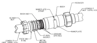
†XJG expansion couplings use a metallic bushing and ground springs to create a high integrity internal ground connection. External ground straps offer a redundant ground path and easy visible indication of ground.
