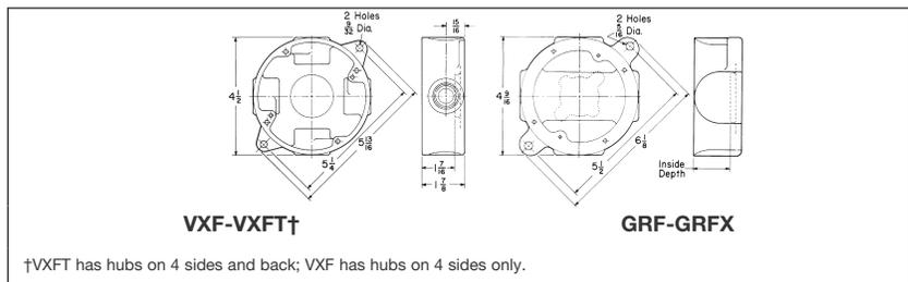
†VXFT has hubs on 4 sides and back; VXF has hubs on 4 sides only.
