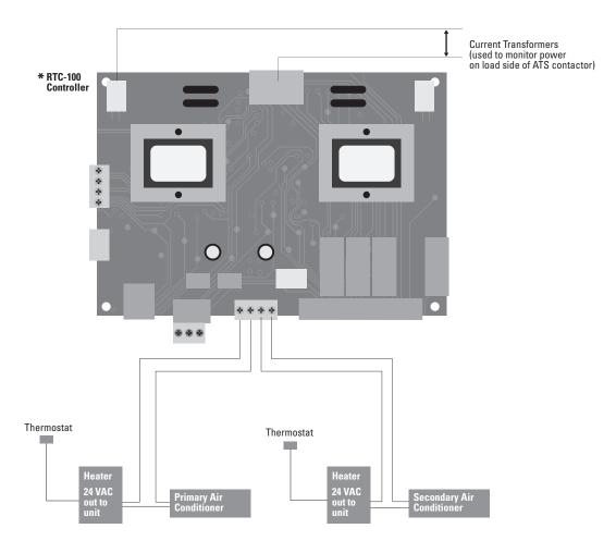
\* RTC-100 Controller is located inside Eaton's Green Line of ATS's.
