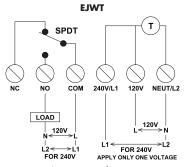
Use copper conductors. For supply connections use AWG #12 wire rated for at least 90°C (194°F) or equivalent.
