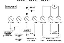
Use copper conductors. For supply connections use AWG #12 wire rated for at least 90°C (194°F) or equivalent.
