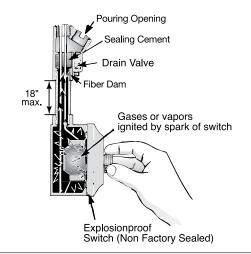
Appleton sealing fittings are suitable for Class I and II locations. EYS, SF and EYD are for sealing vertical conduit. EY and ESU are for sealing vertical and horizontal conduit. SF and EYD also have drain valves.
