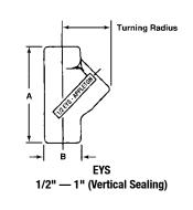
\* Per NEC 501.15(C)(6), seals in Class I, Division 1 and 2 must be limited to conductor fill of 25% of cross sectional area of a rigid metal conduit of the same trade size unless approved for higher percentage fill. See 40% fill sealing fittings. † Turning radius with cover or plug removed.
