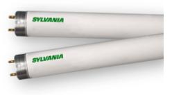
General25W, 36" MOL, T8 OCTRON fluorescent lamp, 4100K color temperature, rareDescription:earth phosphor, 75 CRI, suitable for IS or RS operation, ECOLOGIC
