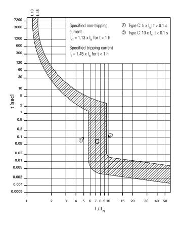
FAZ-NA UL 489 circuit breakers at 480/277 Vac-10 kAIC, 14 kAIC C curve (15-25 A)
