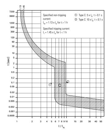
FAZ-NA UL 489 circuit breakers at 480/277 Vac— 10 kAIC, 14 kAIC C curve (15–25 A)
