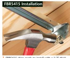
1 FBRS415 ships ready to install with a 1/2" thick ceiling. For a deeper ceiling bend bracket ends along the appropriate score lines as shown at right.
