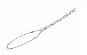
Standard-duty, Closed Mesh, Single eye grip. Cable Diameter - .0500-.0610", Bale length, 7", Mesh length, 11", Break strength, 770 lbs.
