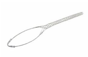
Standard-duty, Closed mesh, Single eye grips. Cable diameter - 0.750-0.990", Bale length - 8", Mesh length - 14", Break Strength - 1,300 lbs.
