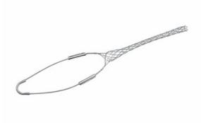
Standard-Duty, Closed mesh, Single Eye Grips. Cable diameter - 1.000-1.240", Bale length - 9", Mesh length - 15", Break strength - 1,680 lbs.
