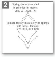
Attach second grille spring to fan and push grille up against ceiling.
