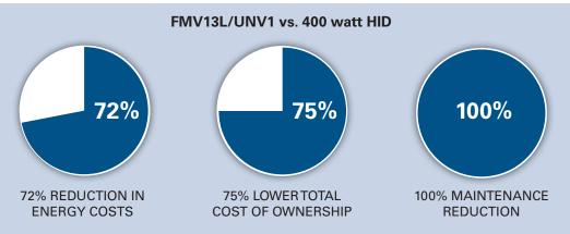
Assumptions: Calculations based on overall life of the LED system. Energy cost of \$09 per kilowatt; 24 hour per day operation; labor rate of \$75 each for 2 workers; average time for fixture maintenance of 1 hour.
