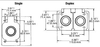
NOTE: All receptacle covers have an overall height of 1.16 in/29.5 mm.
