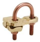
Mechanical Grounding Connector, Conductor to Water Pipe, 4-4/0 AWG, 1/2"-1" Pipe, 3/8" Stud, 3.25 IN Width.
