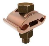
Mechanical Grounding Connector, 2 Cables to 1/4" Thick Bar, 4 AWG (Sol)-2/0 AWG (Str).
