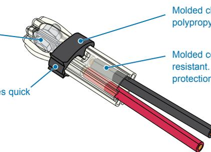
Molded clamp of UV stable, impact resistant polypropylene secures cover in place.
