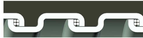
Square-Locked Design with cord packing 3/8" through 1-1/4"
