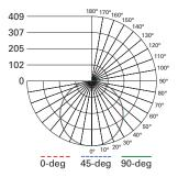
Spacing criterion: (0-180) 1.27 (90-270) 1.27 (Diagonal) 1.39 Beam Angle: 115° Lumens: 1285 Input Watts: 17.24 W Efficacy: 74.6 LPW Test Report: HLCMS9129301EWH.IES
