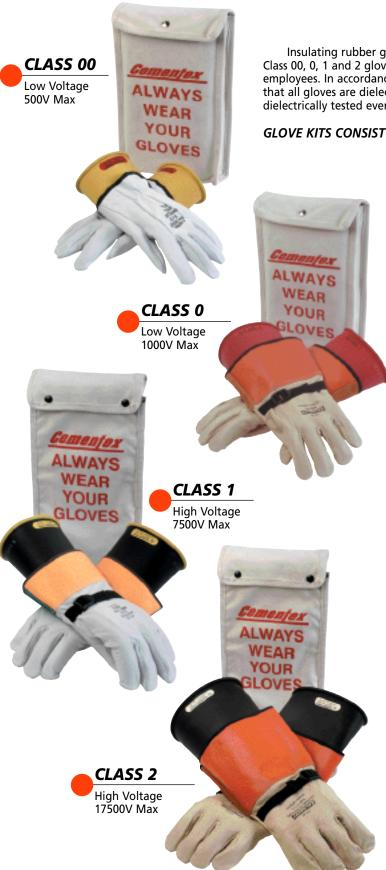
Insulating rubber gloves are the first line of protection against electrical shock. Class 00, 0, 1 and 2 gloves are available in a full range of sixes to comfortably fit most employees. In accordance with OSHA Standard 1910.137(b)(2)(xii) Cementex Certifies that all gloves are dielectrically tested at time of sale. OSHA also requires gloves be dielectrically tested every 6 months.
