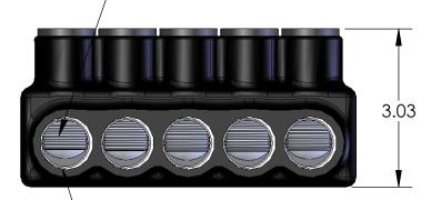
WIRE ENTRY POINT WIRE RANGE: 600KCMIL - #6AWG PRE-FILLED W/ OXIDE INHIBITOR-
