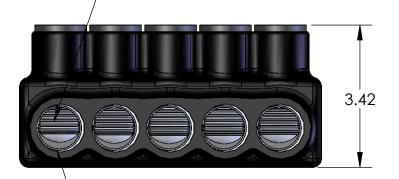
**WIRE ENTRY POINT** WIRE RANGE: 750KCMIL - 1/0 PRE-FILLED W/ OXIDE INHIBITOR-
