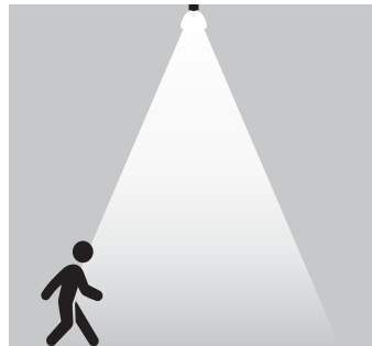
With insufficient ambient brightness, light dims to 100% when motion detected
