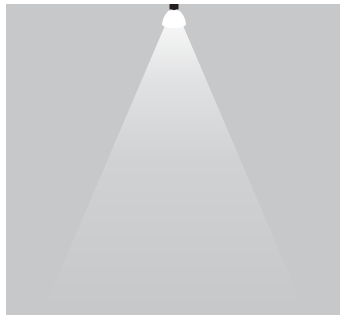
Light automatically on when ambient brightness is lower than preset lux level.
