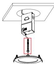
Lifting both retention tabs upward, push the fixture into the hole until trim sits flush with ceiling.
