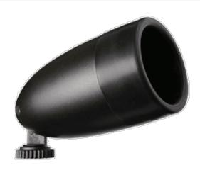
Premium PAR38 Flood with large, molded high temperature black silicone gasket that totally seals lamp. Die cast aluminum housing. EZ Locknut. Suitable for mounting within 4' of the ground. PAR38 or PAR20, 150 Watt max. Lamp not supplied.
