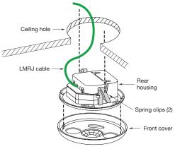
Mount directly to ceiling tile using spring clips (included) or to a 4" octagonal box. See installation instructions for more details.
