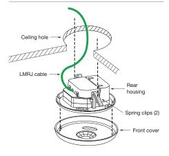
Mount directly to ceiling tile using spring clips (included) or to a 4" octagonal box. See installation instructions for more details.
