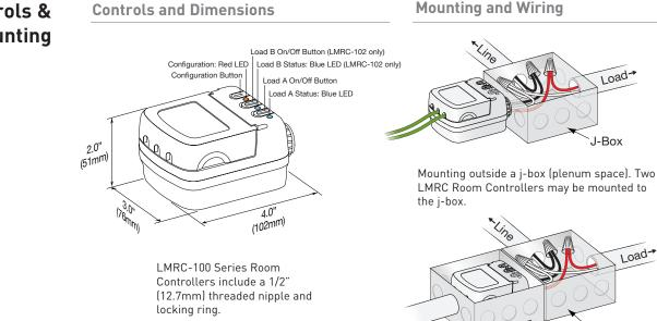
Mounting inside a j-box. Low voltage wiring is run to the LMRC Room Controller in conduit.
