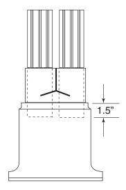
b. Install boot over three phases, resting it on the crotch of the cables (see illustration to the right).
