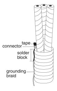
d. Apply two wraps of red mastic around the cable jacket under the solder blocked part of the ground braid, then apply a second wrap of red mastic around the cable jacket and the ground braid. If correctly installed, there should be mastic over and under the solder block of the ground braid (see illustration to the right).
