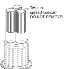
**Partially** remove each leg holdout allowing about 1.5" (38mm) of holdout to remain inside large black plastic body holdout. Do Not Remove Completely.
