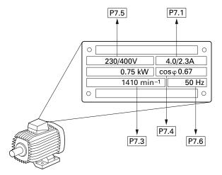
The motor data is set to the rated operation data for the frequency inverter and depends on the performance variables in factory settings.
