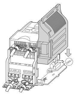
Make the connections to the selected fieldbus system through the opening in the mounting frame directly on the card
