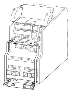
The cable hold down clamps contained in the scope of delivery can be mounted on the cable clamp plate of the power section.
