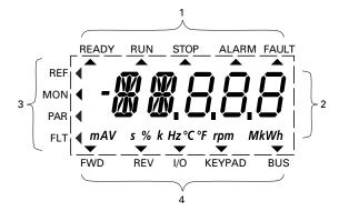
The display unit consists of a backlit liquid crystal display (LCD). It is divided into four areas.
