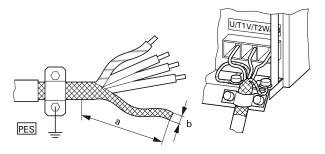
Twisted shielding braid should be connected with a ring cable terminal (see figure on **Page 33**) on PES.
