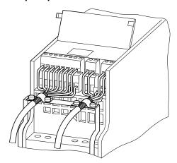
Prevent any unraveling on the other end of the control line with a rubber grommet. The shielding braid is not to make any connection with protective ground here because this would cause problems with an interference loop.
