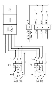
For alternating operation (rotary movement "exclusive or" of the transport rollers) on the rotary table, a frequency inverter for the largest connected load (MMX34AA4D3\_) was selected.
