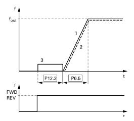
After the time set has elapsed, the frequency inverter starts automatically with the acceleration time set at P6.5. The speed of the motor [2] follows the characteristic of the output frequency [3]
