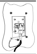
Assemble door panel adapter (item 4) to a cover and UART connector. After that, connect cable (item 3) to door panel adapter (item 4).
