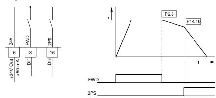
The Stop function with deceleration time can be activated with parameter P6.8 = 1. If the enable signal on the digital input DI1 (FWD, control signal terminal 8) is switched off, the output frequency of the frequency inverter can be reduced according to the deceleration time (dec1) set at P6.6.
