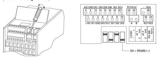
The two control signal terminals A and B enable the connection of a shielded RS485 twisted-pair cable.
