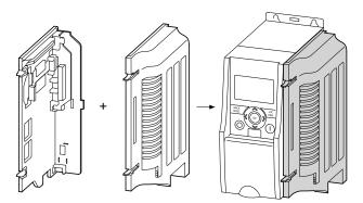
**Note:** The MMX-NET-XA mounting frame is not supplied with the M-Max frequency inverter.
