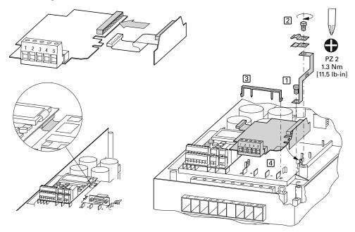
**Note:** Before installing the fieldbus interface card check whether the plug connection provided, such as GND or bus terminal resistor have to be changed.
