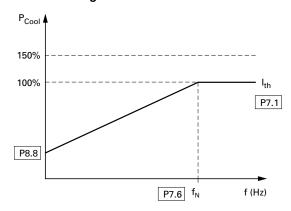
The time constant for the motor temperature (P8.9) defines how long it takes until the temperature has achieved 63% of its end value in the motor. In practice, this temperature time is constant depending on the type and design of the motor. It varies between the different design sizes at the same shaft power and between the different motor manufacturers.
