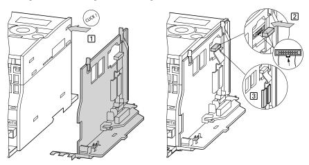
You can then fit a fieldbus interface card (for example, PROFIBUS DP, and so on) in the cover of the mounting frame
