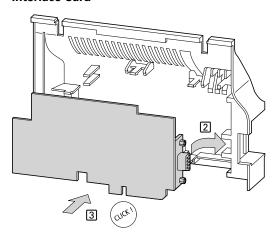
Then fit the cover with the inserted fieldbus interface card onto the already fitted and installed mounting plate of the MMX-NET-XA
