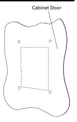
Place the control keypad base (item 1) toward the opening so that the screw holes you made in the cabinet door meet the bushings on the backside of the base. See figures below.
