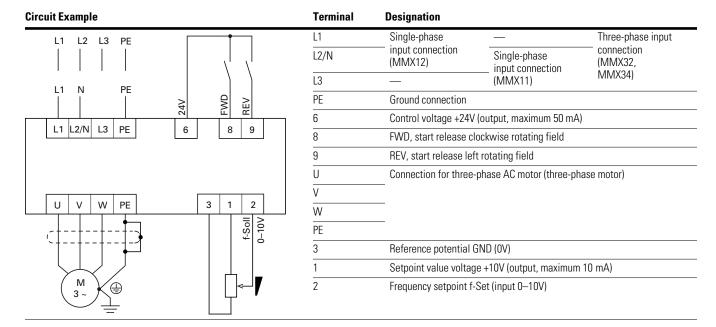
Connect the frequency inverter according to the connection example for simple commissioning with the specified default settings (see connecting example above).
