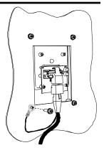
Assemble door panel adapter (item 4) to a cover and UART connector. After that, connect cable (item 3) to door panel adapter (item 4).
