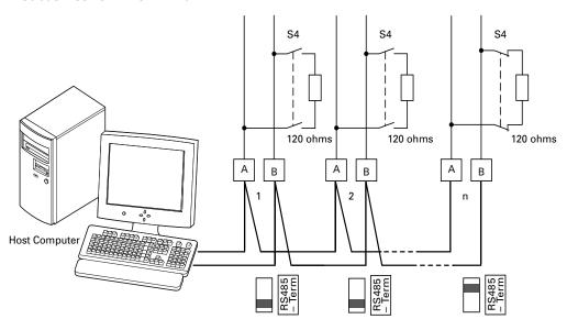
The figures shows a typical arrangement with a host computer (master) and any number (maximum 31 slaves) of frequency inverter M-Max (slaves). Each frequency inverter has a unique address in the network. This addressing is executed individually for each M-Max via system parameter S2.3 and is independent of the physical connection (position) in the network.
