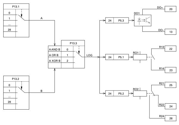
**Example:** Digital output RO1 (N/O contact R13/R14) is required to indicate during operation that the set current limit has been reached:
