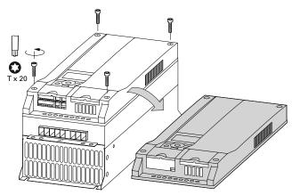
Accessories are provided with the MMX-NET-XB for fitting the fieldbus interface card and interface module.
