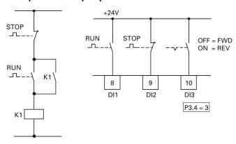
Standard actuation for a drive with pushbutton switch (Normally open, Normally closed) and self-actuating.
