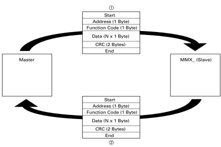
The frequency inverter (slave) only sends a response if it has received a request from the master beforehand.
