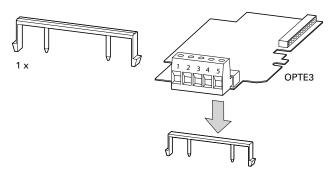
Then connect the required fieldbus interface card to the MMX-NET-XB interface module The mounting is carried out without tools at the corresponding cutouts in the housing of the MMX (snap fitting). Plug and connection cable are then fitted to the interface of the MMX (below the LCD display unit).
