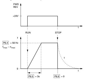
As an alternative (OR) to operation via control signal terminals, you can also operate the frequency inverter without connecting the control signal terminals by simply switching the control level and the setpoint value input.
