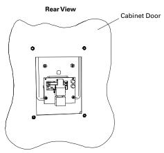
Fix the base on the cabinet door by tightening the screws (item 5).
