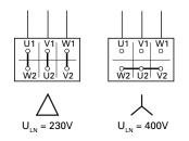
**Example:** Single-phase connection of the MMX12AA4D8\_ frequency inverter to a input voltage of 230V. The stator winding of the motor is connected in a delta circuit (motor rated current 4A as per nameplate in figure on this page).
