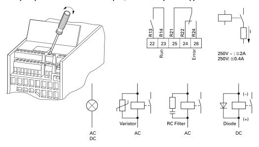
The two relay outputs (control signal terminals 22 to 26) enable the frequency inverter to generate galvanically isolated feedback signals in control circuits with other potentials:
