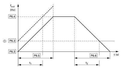
The values for the acceleration time  $t_1$  and the deceleration time  $t_2$  are calculated as follows:
