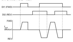
The start enable via control signal terminal 8 (DI1) is always required for operation:
