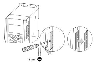
The remaining installation steps are then carried out without any tools using the cutouts provided in the housing of the MMX (snap fixing).
