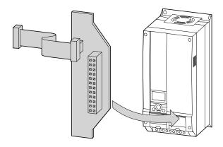
**Note:** The MMX-NET-XB interface module is not supplied with the M-Max frequency inverter.
