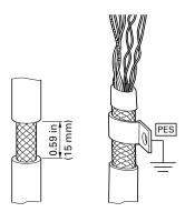
As an alternative, in addition to a broad area cable clip, you can also twist the shielding braid at the end and connect to protective ground with a cable clip. To prevent EMC disturbance, this twisted shielding connection should be made as short as possible (see figure on Page 35).
