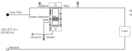
Note: Connect green-sleeved wire to ground only in retrofit and replacement applications.
