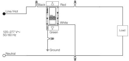
Note: When a neutral connection is available, remove green sleeve and connect the white wire to neutral
