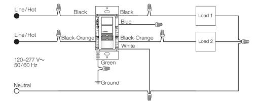
Wiring must comply with NEC<sub>®</sub> code for wiring multiple branch circuits. Where two or more branch circuits supply devices or equipment on the same yoke, a means to simultaneously disconnect the ungrounded conductors supplying those devices shall be provided at the point at which the branch circuits originate.
