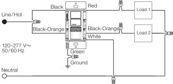
Note: When a neutral connetion is available, remove green sleeve and connect the white wire to neutral.
