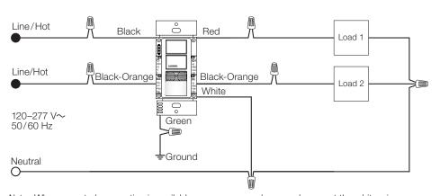
Wiring must comply with NEC® code for wiring multiple branch circuits. Where two or more branch circuits supply devices or equipment on the same yoke, a means to simultaneously disconnect the ungrounded conductors supplying those devices shall be provided at the point at which the branch circuits originate.
