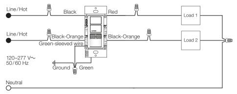
Note: Connect green-sleeved wire to ground only in retrofit and replacement applications.
