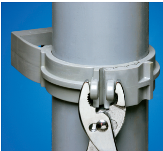
2-1/2" - 4" Press pipe into QuickLATCH, up to the first notch to lock it in place. Finish by squeezing tabs together for a super-secure hold.
