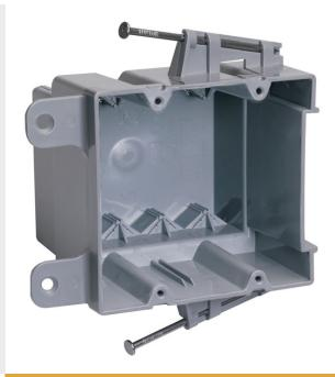
Double Gang, Switch and Outlet box with captive mounting nails on each end. It has four Auto/Clamps on each end. It is made with a durable, impact-resistant thermoplastic box. It is easy to install with a rectangular cutout. 100 pack.
