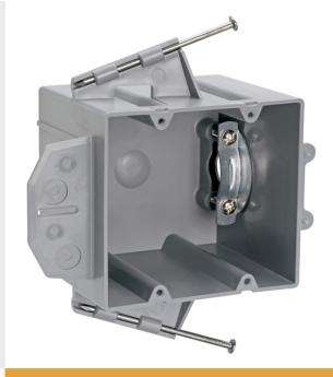
Range and Dryer Box with Captive Mounting Nails on Each End. 1/2" offset for wood or steel stud mounting with metal cable clamp. 12 pack.
