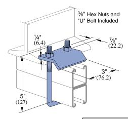
Design Load Each 1000 Lbs (4.4 kN) Use in Pairs Only
